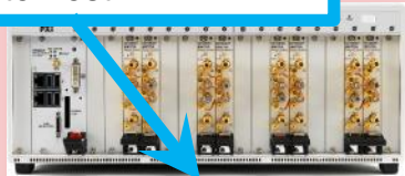
PXI VNA Drive down the size of test 300 k to 26.5 GHz
