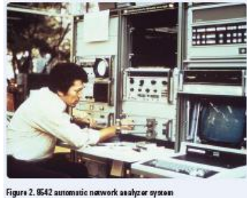
Figure 2. 8542 automatic network analyzer system
